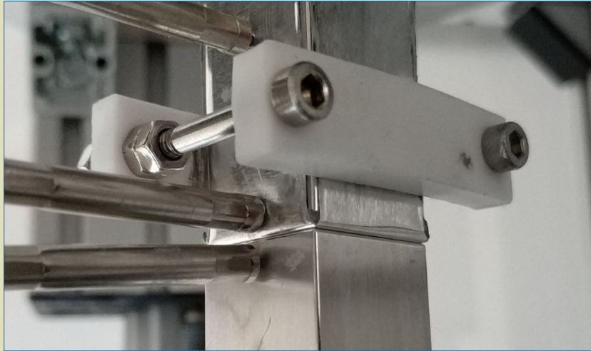
Test heads with aluminum-clad (5 \mu ) flat indium foil TIM2 applied.
