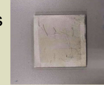
Matte Tin Plate for Tip Contact
