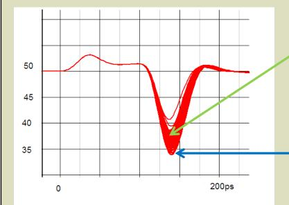
Corresponding time domain reflection measurement set to the S11 solution set
