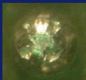
Solder Ball Surface Degraded
