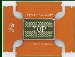
Four wing probe for DDR memory
