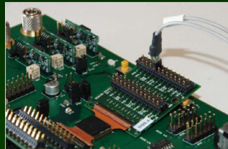
Four wing probe for DDR memory
