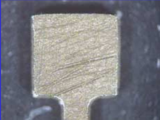
Figure 2. 50 \mu\text{m} thick gold plated conductor pads after 500 hrs at 125 ^{\circ}\text{C} . This is typical of appearance of similar conductor pads.
