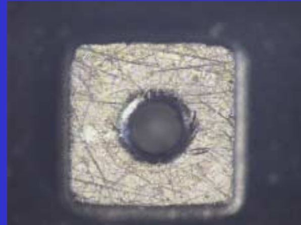
Figure 6. 100 µm nickel plated conductor pad after 1,000 hours at 125°C.
