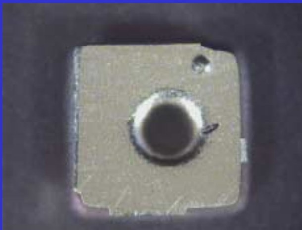
Figure 2. 50 \mu\text{m} thick gold plated conductor pads after 500 hrs at 125 ^{\circ}\text{C} . This is typical of appearance of similar conductor pads.
