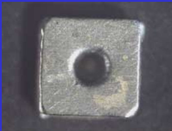
Figure 5. 300 µm thick solder plated conductor pads after 1,000 hrs at 125 °C. Note 5 mil deep witness marks left in the solder.
