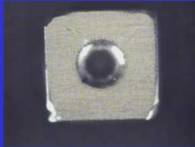
Figure 3. 50 \mu\text{m} thick gold plated conductor pads after 1,000 hrs at 125 ^{\circ}\text{C} . Note good uniform appearance.
